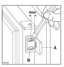
Should the lining up of the furniture door be necessary, use the clearance of slots.
